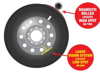
The roller measures the <u>entire</u> contact patch of the tire, detecting if the assembly is out of round.
