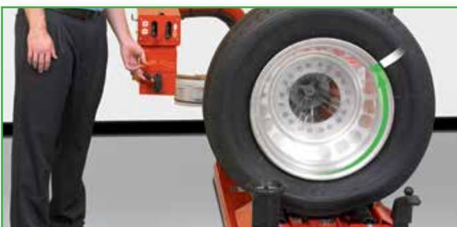
Match-mounting the high spot on a tire to the low spot on a rim makes the assembly roll as smoothly as possible.
