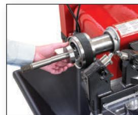
... by loosening clamp screw, removing rotor setup, rotating twin cutter...
