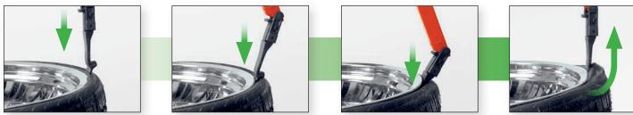
Tool head inserts into tire, pulls bead over and demounts in one fluid down/up motion.
