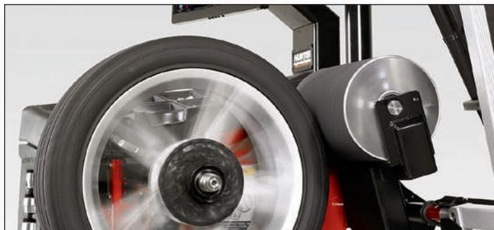
When used with Hunter's Road Force Touch® GSP9700, the Auto34S quickly and easily helps eliminate vibration problems balancers alone can't fix.
